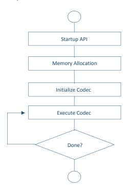
Figure 2 Audio Processing Component Flow Overview
